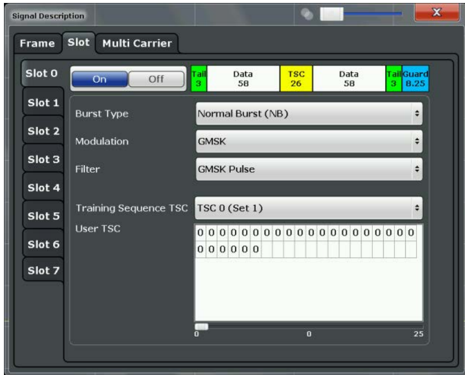
Fig. 6-1: Slot configuration for normal and higher symbol rate bursts
